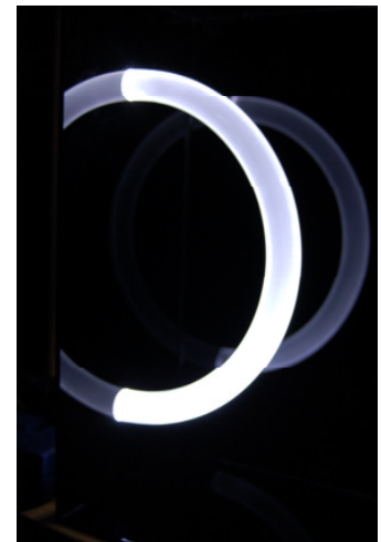
Figure 2: Two-sided lighting of a PLEXIGLAS® EndLighten rod, 20 mm outer diameter with LED light (3x1.5 Volt AAA batteries).
