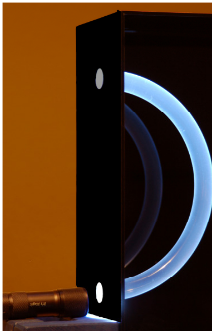
Figure 1: One illuminated side of a PLEXIGLAS® EndLighten rod, 20 mm outer diameter with LED light (3x1.5 Volt AAA batteries). The opposite end of the rod is e.g. laminated with a mirror film to reflect the light. The reflector could also be a bright white PLEXIGLAS®.
