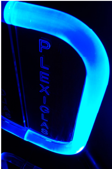
Figure 3: One illuminated side of a PLEXIGLAS® EndLighten rod, 20 mm outer diameter with blue LED, OSRAM DX1-B2-L12W. The opposite end of the rod is laminated with a mirror film. Used PLEXIGLAS® sheet: PLEXIGLAS® Fluorescent 5C50, 3 mm.
